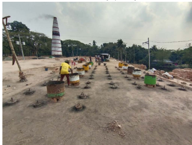
Fig. 1. Key intervention practices. This figure depicts the standard brick setting and fuel feeding practices and the changes proposed in the intervention. (A) The standard zigzag kiln brick setting practice in which brick columns are packed densely with a single zigzag airpath. (B) The intervention recommended practice of less dense brick setting with two or three zigzag air paths. (C) The standard fuel feeding practice of several firemen feeding simultaneously during intermittent feeding intervals. (D) The improved practice of individual firemen feeding fuel continuously in shifts so that there is no pause in feeding overall. More details on the intervention can be found in the full materials and methods in the SM.
