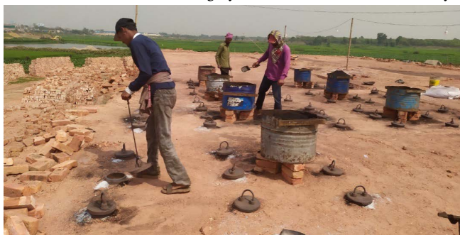
Fig. 1. Key intervention practices. This figure depicts the standard brick setting and fuel feeding practices and the changes proposed in the intervention. (A) The standard zigzag kiln brick setting practice in which brick columns are packed densely with a single zigzag airpath. (B) The intervention recommended practice of less dense brick setting with two or three zigzag air paths. (C) The standard fuel feeding practice of several firemen feeding simultaneously during intermittent feeding intervals. (D) The improved practice of individual firemen feeding fuel continuously in shifts so that there is no pause in feeding overall. More details on the intervention can be found in the full materials and methods in the SM.
