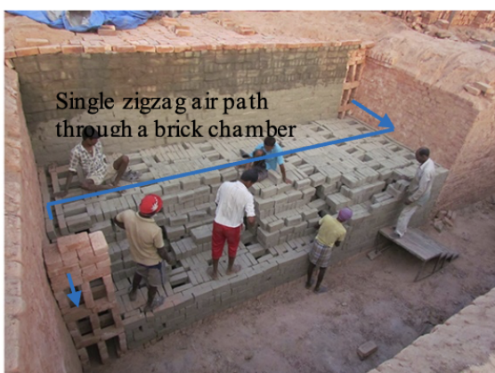
Fig. S5. Dense zigzag brick stacking with single zigzag path. This picture shows the standard dense brick setting practice (left) and the resulting airflow in a single zigzag path. See Technical Intervention Details for details.
