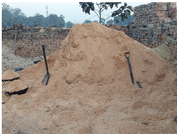
Fig. S10. Sawdust for feeding in newly inducted chambers in the fuel feeding zone. This picture depicts the practice of using sawdust in the front chambers of firing, as recommended by the technical intervention. See Technical Intervention Details for details.
