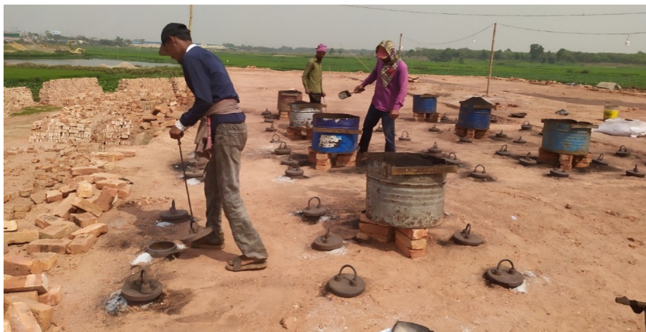
Fig. S7. Intermittent fuel feeding by 2 or 3 firemen simultaneously. This picture shows the standard practice of 2-3 firemen feeding coal simultaneously into the kiln. See Technical Intervention Details for details.
