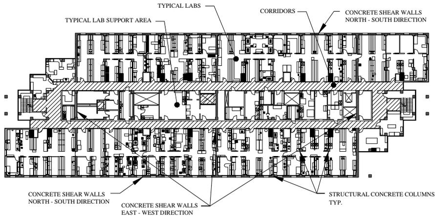
**Figure 2 Typical Floor Plan 2<sup>nd</sup> through 5<sup>th</sup> Floors**
