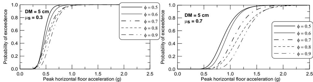
**Figure 4 Sample probability of small equipment exceeding displacement of 5 cm, given a range of  $\phi$  values and: (a)  $\mu_s = 0.3$  and (b)  $\mu_s = 0.7$  [9]**
