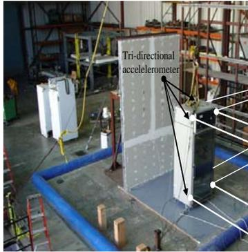
Figure 5 Heavy Equipment on the Shake Table at U. C. Berkeley
