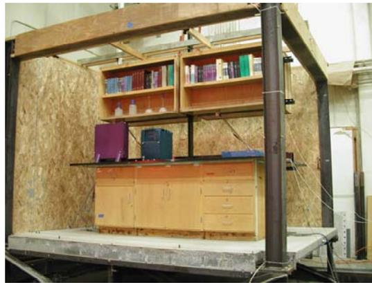
**Figure 3 Bench and Shelf system on the Shake Table at U. C. Irvine**
