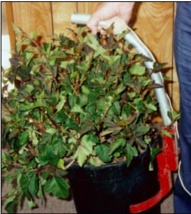
Handle developed by U.C. Davis researchers for carrying nursery containers.
