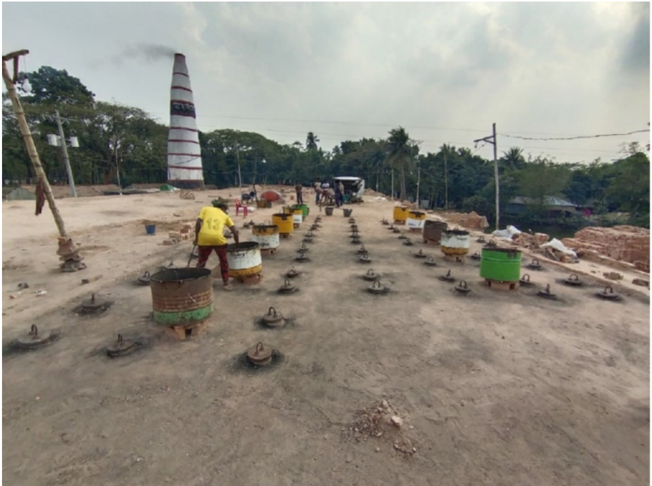
Fig. S8. Continuous fuel feeding by a single fireman. This picture shows the practice recommended by the technical intervention of a single fireman feeding coal. See Technical Intervention Details for details.
