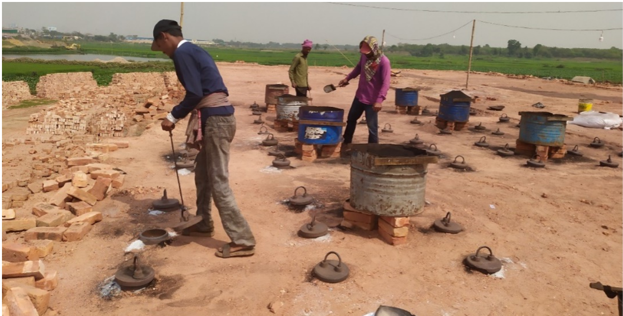
Fig. S7. Intermittent fuel feeding by 2 or 3 firemen simultaneously. This picture shows the standard practice of 2-3 firemen feeding coal simultaneously into the kiln. See Technical Intervention Details for details.
