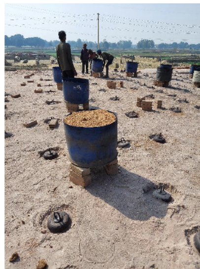
Fig. S10. Sawdust for feeding in newly inducted chambers in the fuel feeding zone. This picture depicts the practice of using sawdust in the front chambers of firing, as recommended by the technical intervention. See Technical Intervention Details for details.
